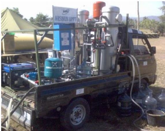
Gambar 14. Arsinum kapasitas 30 m<sup>3</sup>/hari (Genset 1,5 KW, Pompa, Pasir, Cartridge Filter, Ultrafiltrasi, UV Light, Ozonator).
