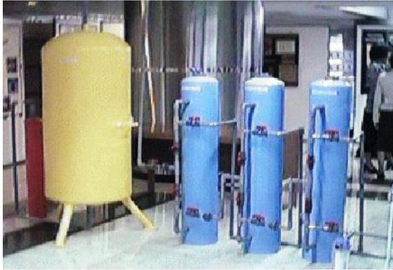
Gambar 13. Filter bertekanan filter multimedia kapasitas 120 sd 160 m<sup>3</sup>/hari.
